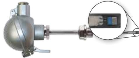
Resistance thermometers are manufactured according to DIN EN 60751 and are available in two-, three- or four-wire technology. Models with two or more measuring circuits are also possible.
